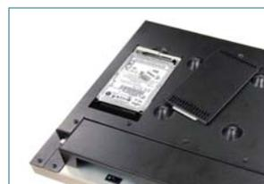
5. Slim HDD bay design for easy service and built-in speakers, and cable cover (option)
